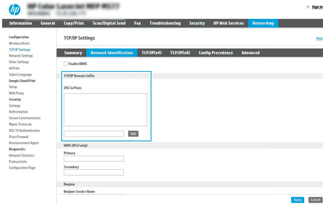
The screenshot shows the HP EWS interface for TCP/IP Settings. The 'Network Identification' tab is selected. A blue box highlights the 'TCP/IP Domain Suffix' section, which includes a 'DNS Suffixes' list and an 'Add' button. Below this, there are fields for 'WINS (IPv4 only)' Primary and Secondary, and 'Bonjour Service Name'. The 'Apply' and 'Cancel' buttons are at the bottom right.
